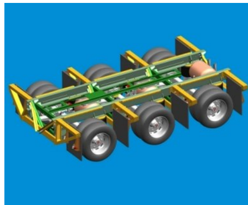
Lightweight wheel section of the GIGA trailer, developed using vacuum infusion, saving hundreds of kilos of weight while reinforcing the structure
